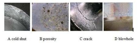
Figure 1 Defects in aluminum alloy castings [9]
